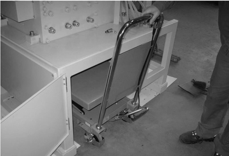
4. Loosen the bolts "A" (4 x silver allen bolts M20 each on front and 4 x silver allen bolts M20 on the back side of the cutting unit
