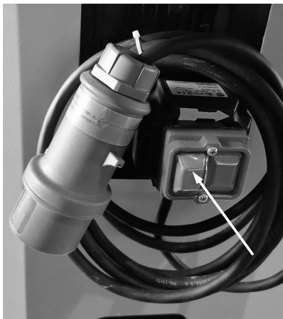
When you press the green button at the dust extractor and leave it pressed, the dust extractor will start automatically when you start the shredder and will stop automatically, when you stop the shredder.
