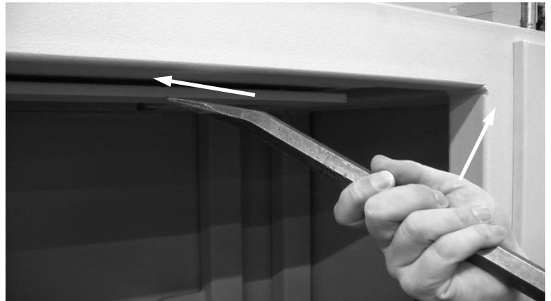
7. Once the screen is sitting on the platform lift, pull it out from under the shredder and remove all magnetic parts from accessible areas underneath the cutting knives and from the screen surface with suitable tools like heavy duty pliers. Also unblock the screen holes with a suitably sized punch. Be careful not to damage the screen.
